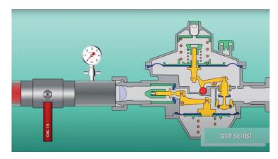
Before commissioning the regulator, ensure that the pipeline connections are made correctly. The inlet and outlet valves should be closed.
