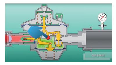
Slowly open the inlet valve, turn the knob on the regulator slowly to allow gas to enter, and release the knob. The regulator will automatically adjust itself once gas enters it.
